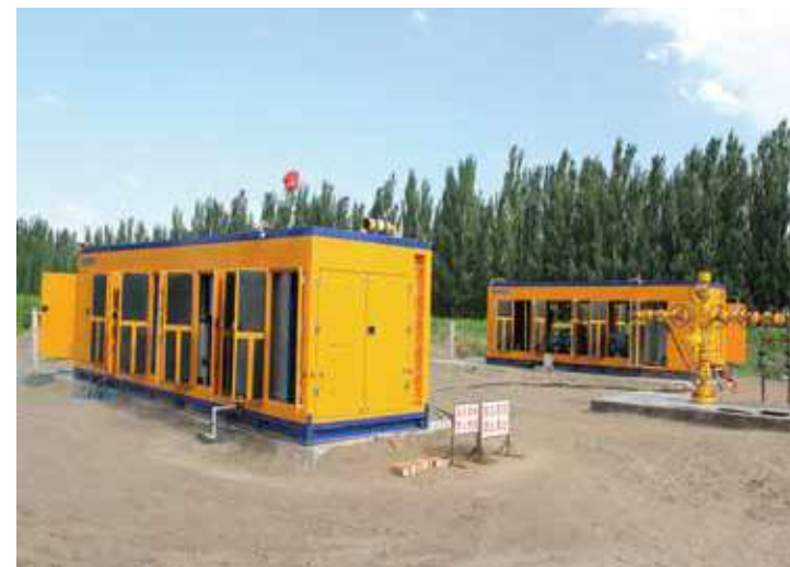
○ China XinJiang 1800 cubic meter 50MPa High pressure Membrane Separation/PSA Nitrogen Generation equipment working site
