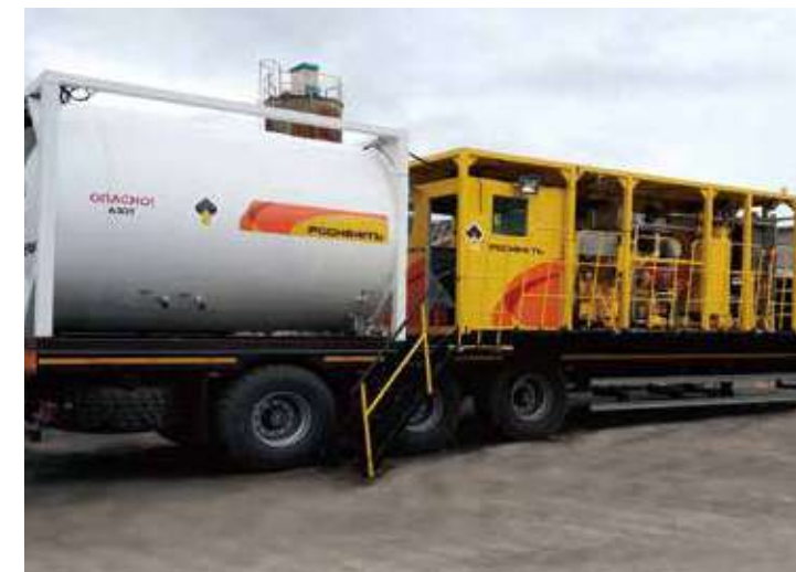
○ Russia LNP-180K/70Q High cold liquid nitrogen pump working site
